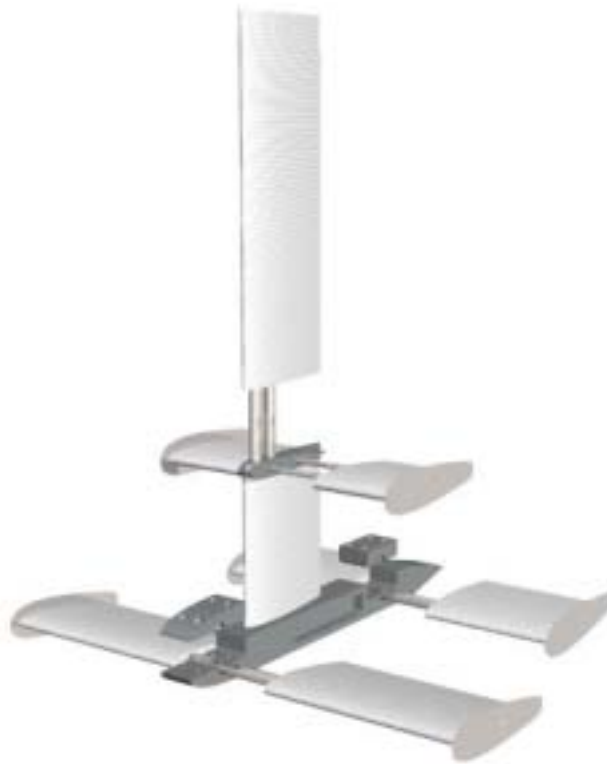
Figure 8.1 – A partially exploded view of the final design - foil assembly for the prototype
