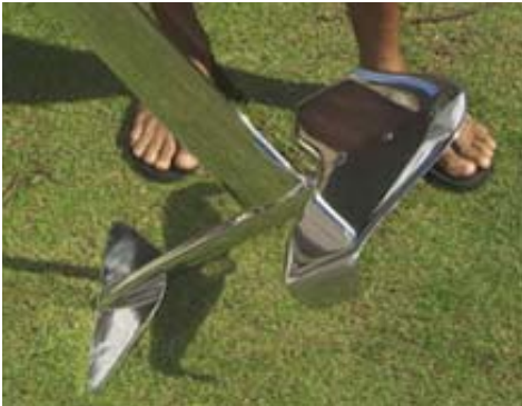
Figure 5.4 A modified version of the Airchair foil, showing the foil assembly and detail of the turned down wingtips used for reducing wingtip vortices. [i10]
