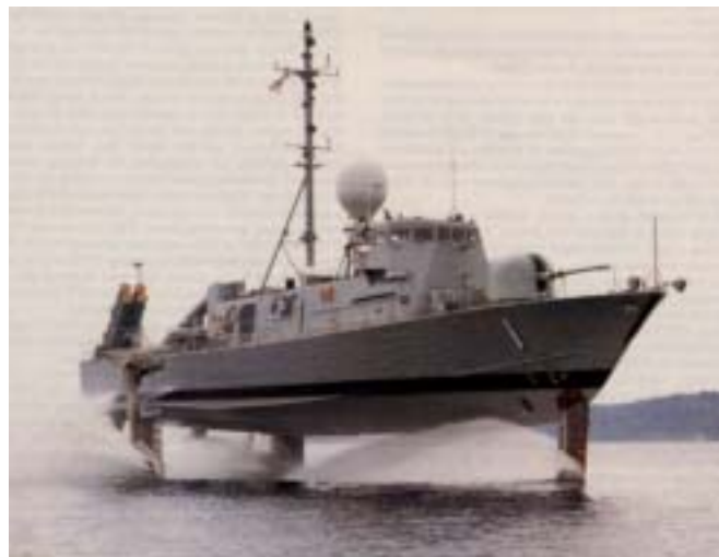
Figure 1.4 USS Pegasus (PHM-1) US Navy Patrol Combatant Hydrofoil - Missile built by Boeing Marine, launched Jun 74; first foilborne flight Feb 75; commissioned into service Jul 77.
