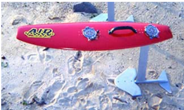
Figure 5.2 Left: An example of a Foilboard, showing the two triangular foils at the base of the main strut
