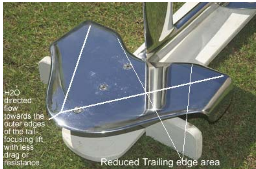
Figure 3.5 – The company offered explanation for the fluid mechanics principles behind the successful functioning of the foil [i9]
